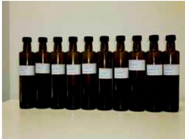
Figure 3.1 Samples stored in dark bottles, prior to storage in a dark cupboards to exclude light
